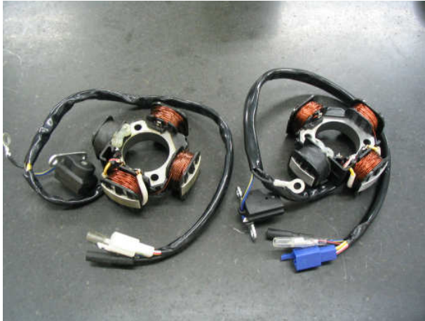
Picture 1 : original stator (white color plug)
