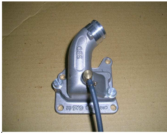
Picture 10: new intake pipe assy.(part no. 421001A ) including an new oil tube (part no. GA605PP02)
