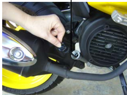
LUBRICATE OIL TANK
