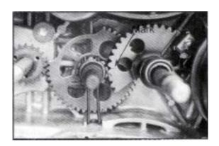
(4) Use special tool for starter arm spring assembly. Rotate tool clockwise, such that spring locking pin is positioned under crank case half-moon location, then assemble stop plate.
