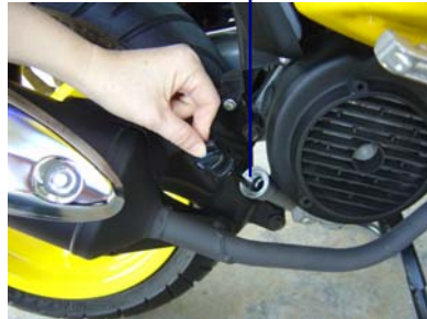
LUBRICATE OIL TANK
