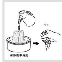
Use solvent for cleaning filter cartridge sponge
